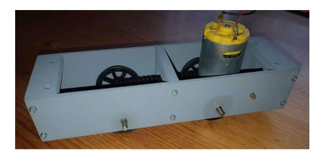
The chassis is built up from a combination of laser cut acrylic sheet and 3D printed parts. The whole assembly is secured with nuts & screws and can be assembled and disassembled to allow for painting and maintenance.
