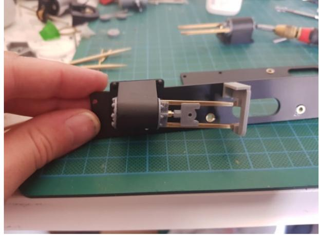
Next remove the cylinder from the frame take the connecting rod and countersunk the small end then fit to the cross-head with a 2mm x 6mm long bolt and nut do not tighten leave loss to float about again make sure it moves freely
